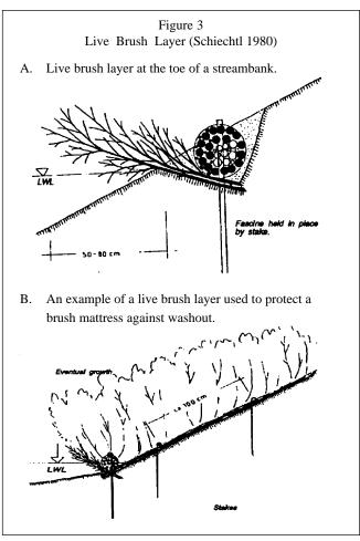
Cuttings may also require protection from flowing water before they can become established. For this reason, cuttings are often incorporated into various bioengineering techniques. Finally, cuttings do not compete well with existing vegetation, and in dry climates follow-up irrigation is required to promote rooting.
