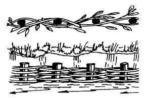
B. Spiling used in conjunction with placement of live cuttings and protective fencing.
