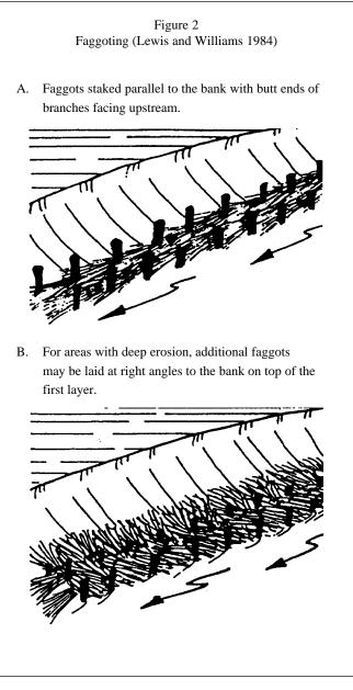
from wave wash. The fascines eventually root and grow, strengthening their effectiveness. Fascines are primarily used in conjunction with other techniques such as brush mattresses, brush layering, branch packing or live siltation fences. In each of these methods, fascines and stakes are used to secure branches placed under them, especially in areas where rocks or other suitable anchoring material is unavailable.
