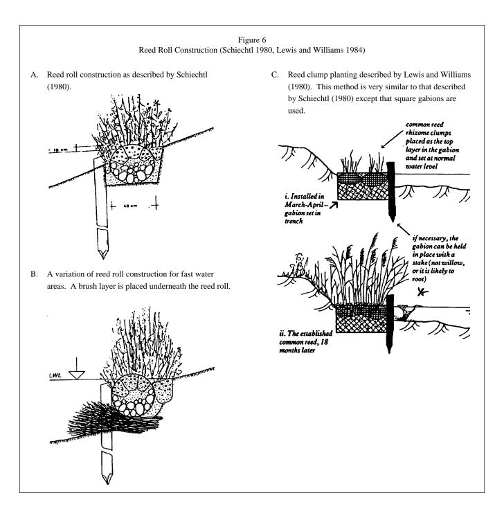
rock gabion on the river side of the reed roll. Reed rolls should be checked occasionally, particularly after floods, to correct any movement. They are also prone to damage from beaver and muskrat, and may need to be isolated by fencing if such damage is occurring.
