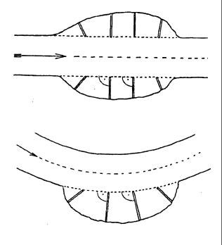
a bank. Construction of these barriers is labour intensive, and limited to a period when parent stocks for branch cuttings are dormant and water levels are low. Also, the need for a final rock layer requires that rocks be available, and their placement may require a backhoe or other heavy machinery.
