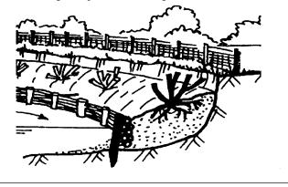
the integrity of the wire mesh is lost before vegetation can establish itself, the new bank may be subject to sudden failure.
