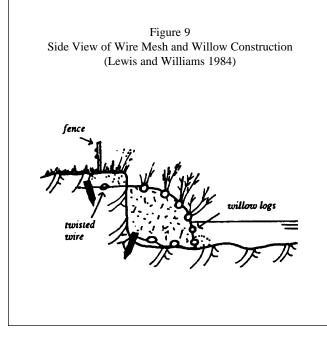
re-establishment of plants, as well as protecting recently planted vegetation. Live siltation barriers are effective immediately upon placement and protection increases as vegetation in the barrier becomes established. Live siltation resists high flows and is inexpensive to construct, usually 1/50 to 1/100 the cost of conventional engineered structures such as dykes and jetties (Schiechtl 1980).
